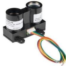
Figure 1. LIDAR-Lite v3 sensor
